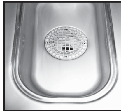
Place pump intake strainers in position at the bottom of wash tank (rinse section).
