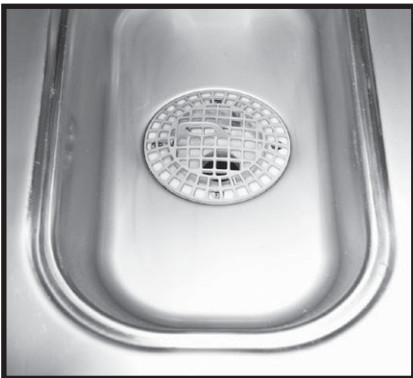
Remove pump intake strainer (rinse section).
