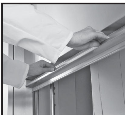
Close inspection doors. Ensure sufficient detergent and rinse aid is available in the right containers.
